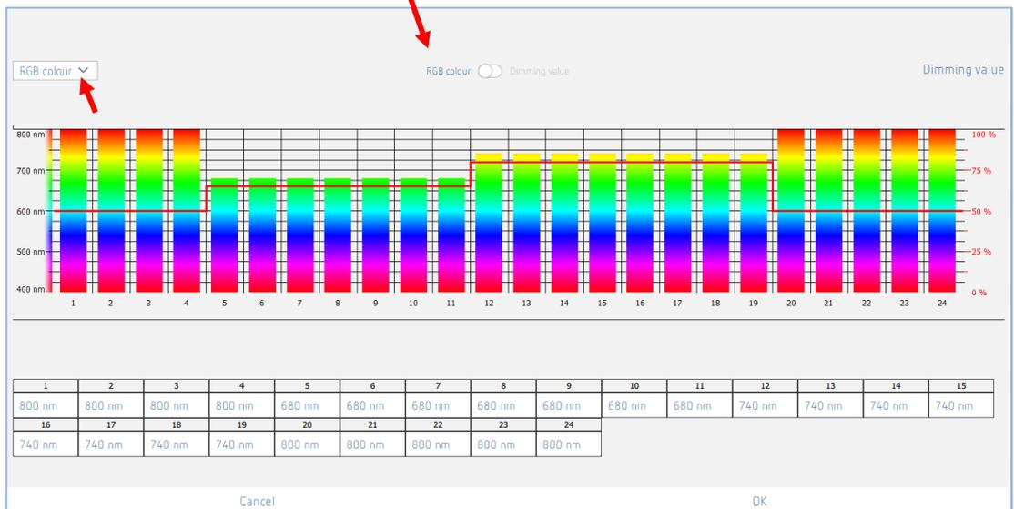
The drop-down menu can be used to switch between the RGB colour curve and the white component curve:
