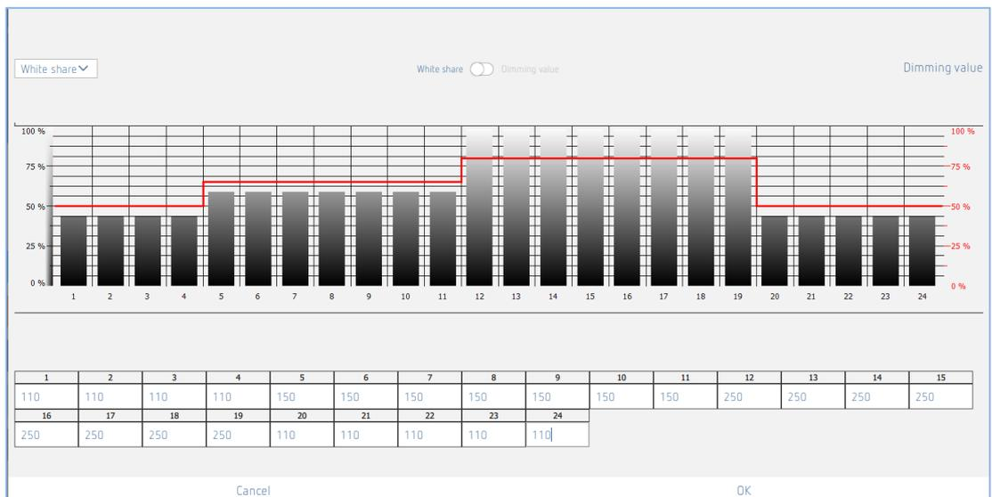
The colour gradient or white component gradient and the dimming values are set as desired by dragging the bar in the diagram or by entering the values in the table.
