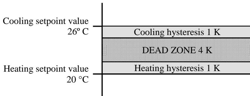
The dead zone (4 K) is increased by the value of both hysteresis (2K) and offsets the cooling setpoint value to 26 °C.
